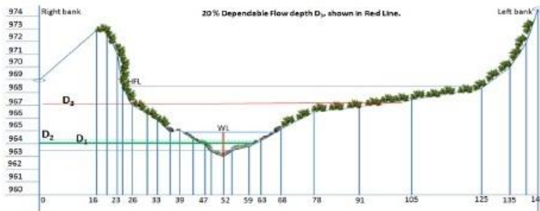
Figure 5.5: River Cross-section at Ranari, Dharasu
